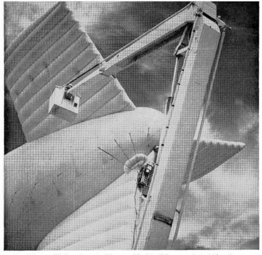
TAIL SECTION of balloon is serviced by a mobile "giraffe" at test site in Idaho. One man in the bucket section operates the boom controls while the second man adjusts the balloon's electrical blower system. Each fin is about 39 feet high.
